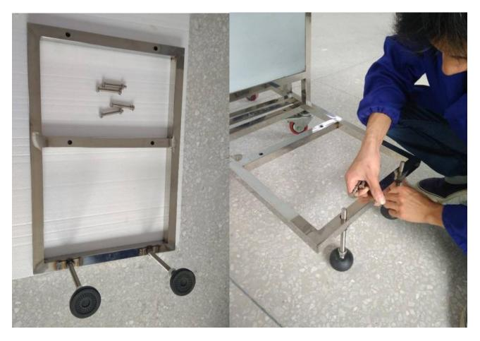
The four holes in the holder are respectively aligned with the four holes in the bottom of the cart. Four screws are inserted into the holes and tightened with a wrench in the part bag. Adjust the support screw so that the holder is firmly supported on the ground. Note that the cart holder must be installed first, otherwise the cart will be dumped.
