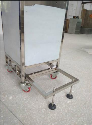
Installation of lifting frame brackets.
