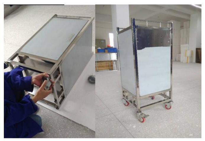
1. Install the four castors in the four nuts on the bottom of the cart.
