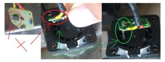
Note: Operation after power off . The circuit board between the two black plastic sheets cannot be removed, and the circuit board must not be wetted. After cleaning the flowmeter impeller, the components of the circuit board need to put as they were
